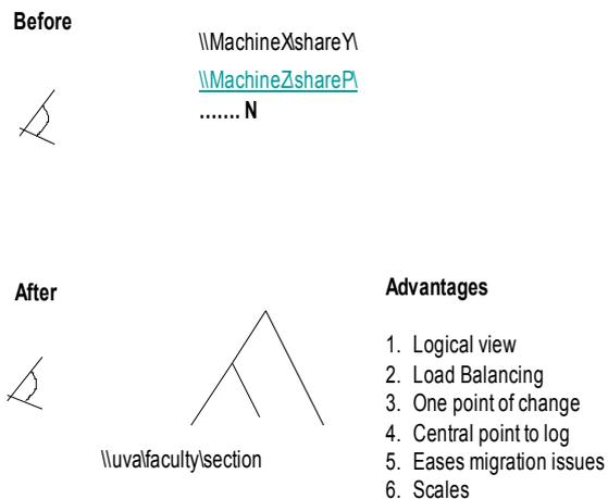
Figure 4: Describes how DFS brings a logical structure to a potentially disjointed physical infrastructure.
