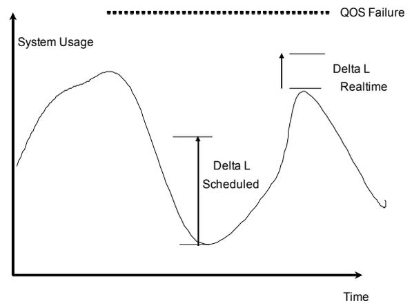
Figure 8: System usage against time showing the effect of load due to real time and scheduled virus checking.
